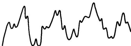
Fig. 303. Noise is characterized by its random irregularity.
