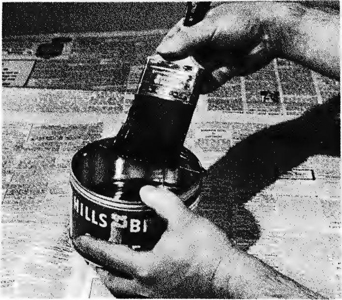
Fig. 707. Technique used when applying lacquer with a brush: a) remove excess lacquer from the brush to aid in producing an even spread; b) apply lacquer in direction of grain. Note the proper way to hold the brush.
