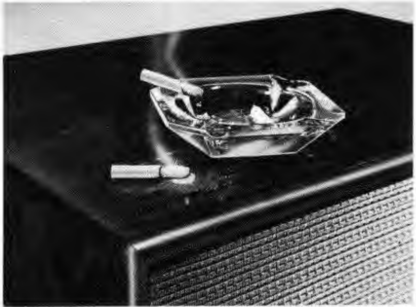
Fig. 801. Most cabinet burns are caused by cigarettes.
