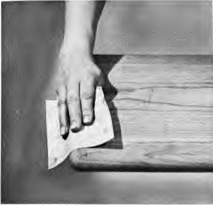
Fig. 703 (continued). This photo shows hand-finishing of curved end using 6/0 sandpaper.
